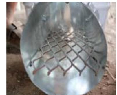
7) Cut a long metal slice; make it together in the ends and put it on the top of the cooker.
